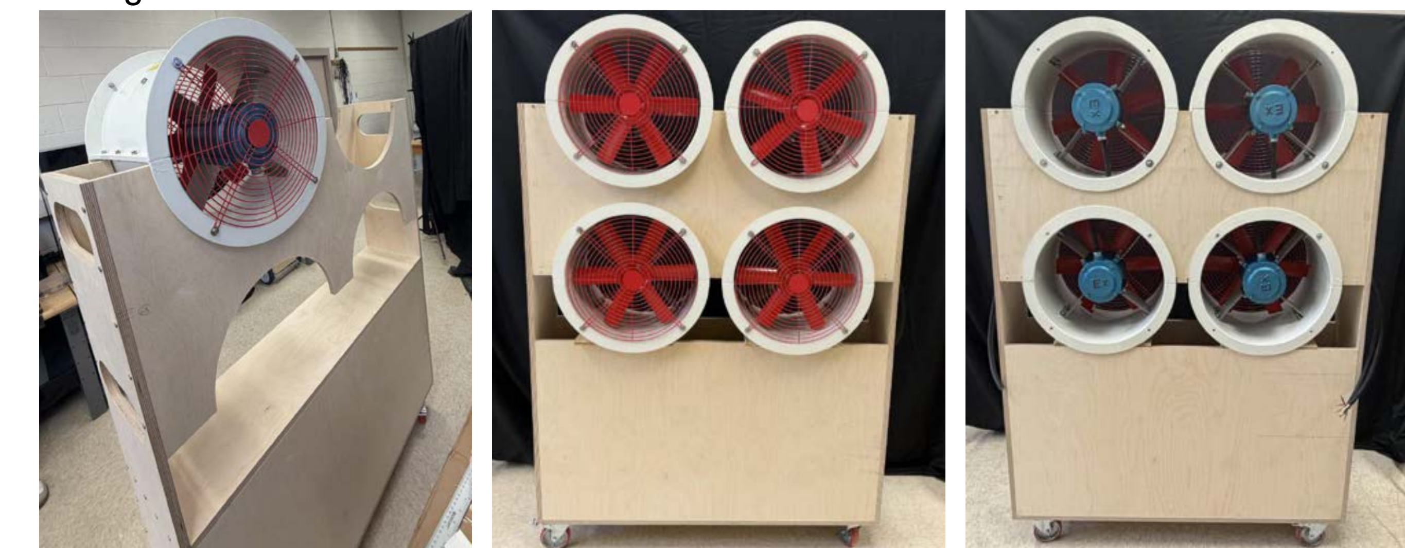
Figure 5. New Fans Mounted in the Custom-Built Baltic Birch Frame
